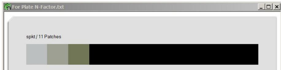
**Please note you can also measure each of the three patches more than one time:** For example, you can measure 3 times the 0% patch, 4 times the 50% patch and 2 times the 100% patch (Maximum total 11 measures, in any order). In this case **PLATE** application will average your measures for computing the **N-Factor**.
